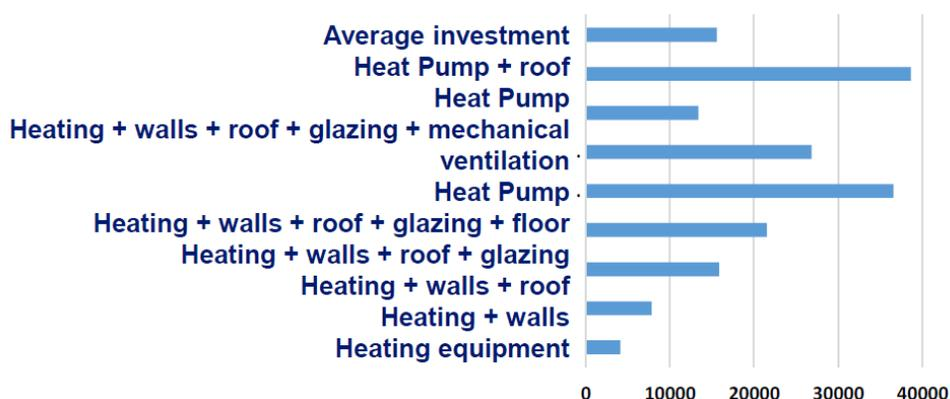
Figure 6. Investment costs for packs of unitary retrofitting actions (equipment + installation, € ex VAT, based on costs/m<sup>2</sup>, source: Osso et al. 2017)
